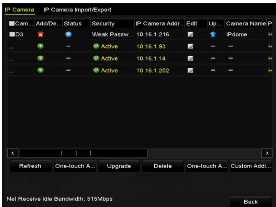
Figure 2. 23 Successfully Added IP Cameras
